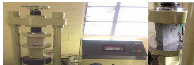
Figure 3 Test Specimen of Compressive Strength Test
